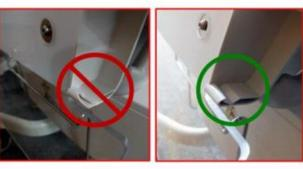
Figure 1C - Broken Latch
